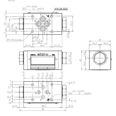
All stackable valves AM3 -\* conform with ISO and CETOP specifications for mounting surface dimensions. Valves height 40 mm. Leakage between valve and mounting surface is prevented by the positive compression on their seats of 4 seals of OR type. All valves have on their "mounting" surface a  $\varnothing$  4 mm cylindrical hole and have on their "seals" surface a  $\varnothing$  3 mm cylindrical hole, conform with ISO and CETOP norms.
