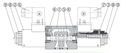
The spool 5 shifts into the valve body 1 subject to the actiong springs 4 and solenoids 9. Spool 5 depending from its shape and its position in the valve body 1, opens and/ or closes passages between P,A,B and T ports, thus controlling the direction of the hydraulic flow.
