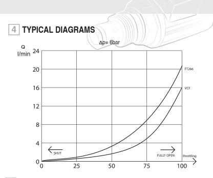
Typical Q curves a different throttling sections and fixed  $\Delta p=6$  bar for valves FT266/VCF. Standard configuration with mineral oil at 42cSt and 50° C.
